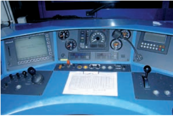
The cab of an ETCS-equipped Vossloh G2000 locomotive.
