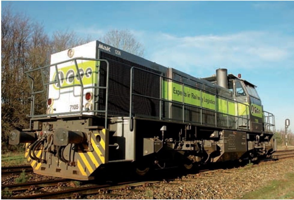
This Vossloh G1206 operated by Dutch open-access company ACTS is equipped with ETCS Level 2 for use on the Betuwe Route.
