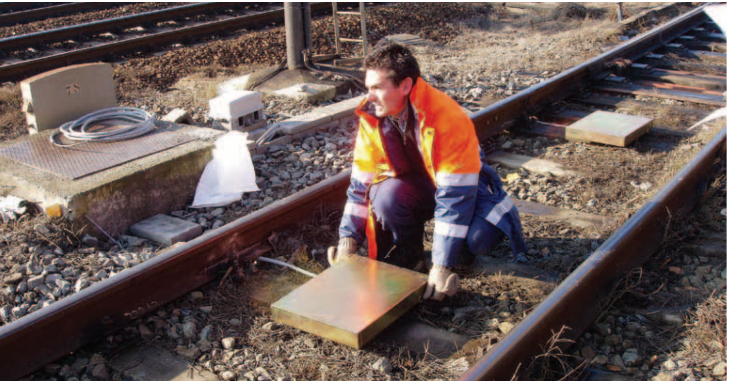
Testing an unshielded balise. The Italians are now looking at radio infill as an alternative to balises for Level 1.
